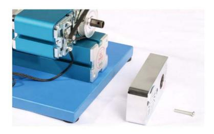
把砂轮安装在主轴上并用内六角扳手拧紧砂轮上的回紧定螺丝。 Install the grinding wheels on the bearing and tighten it.
