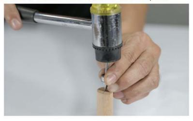
把驱动中心器安装进锣床并用顶尾座把木棒后端顶住。 Place the workpiece between the drive center and tailstock and tighten it. Make sure centers are aligned.
