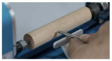
摇动大滑块组件的手柄即可把支撑器左右移动到需要的地方。 Rotate the handwheel to control the slide and position the strutting piece in the right place you need.
