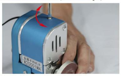
用手压下皮带,皮带压下量为3至5mm时皮带松紧度适宜。 To check the tightness of the drive belt as shown in the figure.
