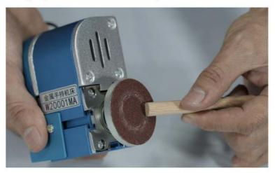
更换打磨头时,使用螺丝刀插入主轴箱尾部,把转盘拆卸。 To change the grinding accessories, use the screwdriver to put through a hole on the end of spindle and twist the grinding wheel.
